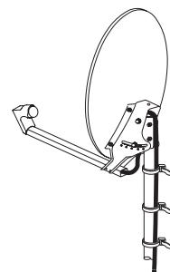
**Note:** If used, the metal pole should have an outside diameter of approximately 1 5/8 inches (approx. 4 cm), and should be sturdy enough not to flex in high winds. If the clamp ends up being slightly loose, use weather proof sandpaper or emery cloth to shim the clamp, and tighten.
