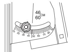
If you have the bracket where the edge of the mast shows through the curved slot, align the edge with the desired elevation mark.
