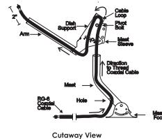
13. Loop the end of the cable over the pivot bolt.
