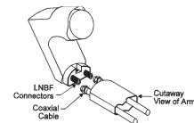
18. Fit the LNB onto the end of the dish support arm, sliding it until it is inserted firmly. Attach LNB to the support arm using the LNB screw and washer.
