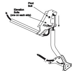
10. Turn the antenna mount on the mast or pole to align the LNB support arm in the direction of the satellite. Use the direction you found earlier in the Satellite Location Reference Chart.
