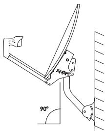
The figure above shows how you should attach the mast to the foot for mounting on vertical surfaces.
