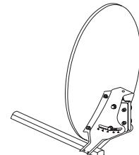
8. Tilt the support bracket to the approximate elevation of the satellite. Use the elevation you found earlier on the Satellite Location Reference Chart.
