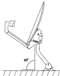
The figure above shows how you should attach the mast to the foot for mounting on horizontal surfaces.
