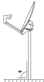
The figure above shows how you should attach the dish support and bracket to a mounting pole.
