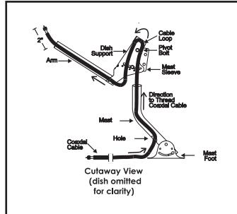
**The assembly and mounting of the 51 cm Dish is complete.
