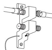
**Grounding Block with LNB Cable**
