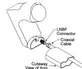
17. Attach the LNB to the LNB cable(s). Slide the weather boot up securely to cover the cable/LNB connection at the base of the LNB.
