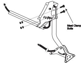
11. Thread the LNB cable into the cable hole near the mast foot, up the mast and out the top of the mast.
